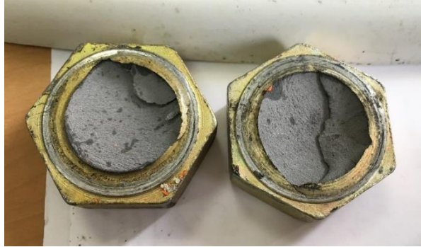
Figure 19. Fracture surfaces of severed bolt heads.
