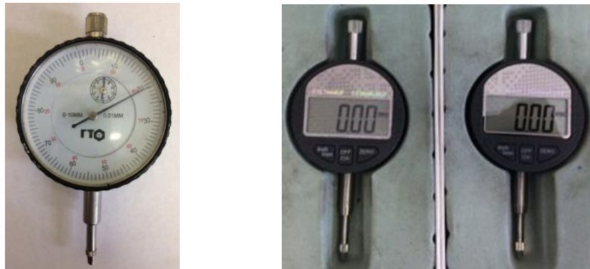
Figure 6. The indicator of hour type ICH-10 and mechanical measuring sensors ICH-10 of hour type.
