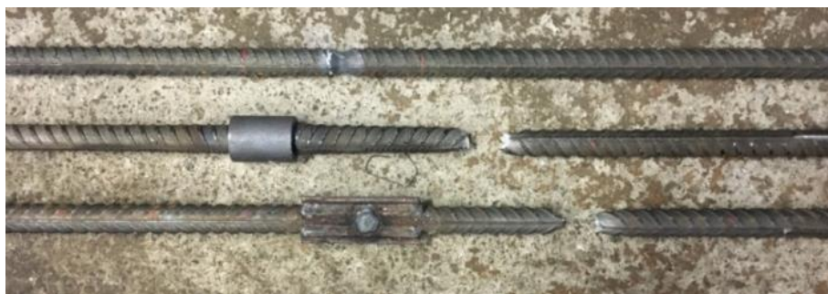
Figure 11. Places of rupture of samples after the 3 rd experiment.
