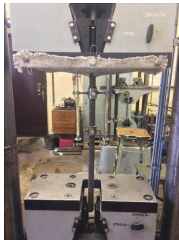
Figure 7. Installation of the sample in the measuring machine.
