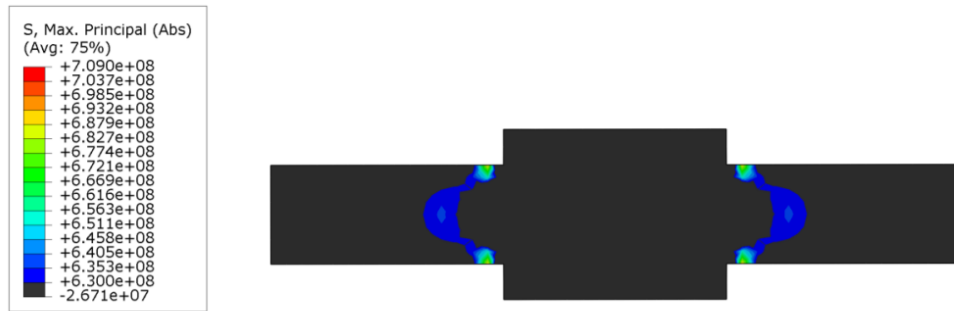
Figure 14. Fracture zone at 200°C.
