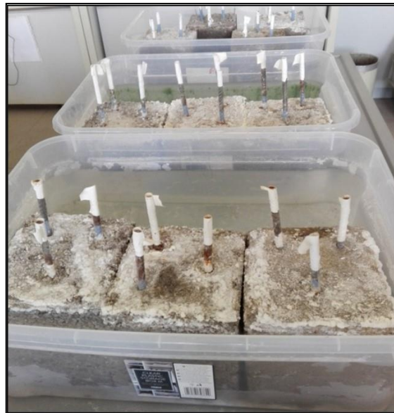
Figure 2. Reinforced concrete samples were immersed in 3.5 % NaCl solution for 18 months.
