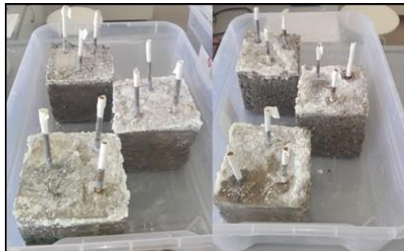
Figure 3. Reinforced concrete samples removed after 18 months immersion in 3.5% NaCl solution.
