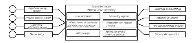
Fig. 1. Functional structure of the automated system "Accounting of material flows" of the metallurgical shopfloor of the Copper Plant
