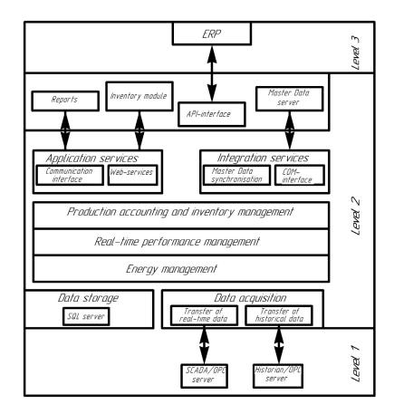
Fig. 3. The generalized structure of the project of the automated material flow management system, planned for further integration into the unified information system of the company "Silarus": level 1 – process control; level 2 – operational production management; level 3 – strategic enterprise management
