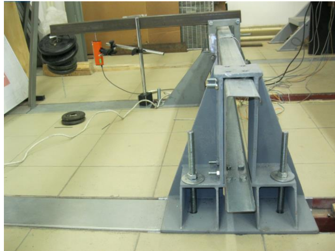
Figure 2. Warping torsion of cold-formed C-shaped steel bar. Joint type 3.
