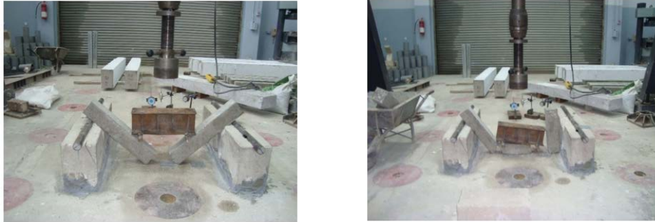
Figure 12. Plain concrete beams failure modes.
