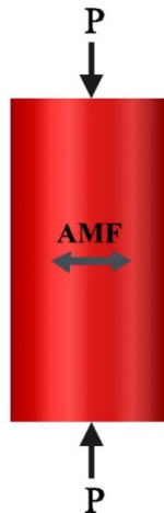
Figure 6. The direction of magnetization of PrM specimens.
