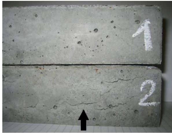
Figure 3. Samples of concrete after low-heat steaming treatment with different duration of preliminary exposure (sample 1 after treatment with mode of 3-3-5-1/40 °C, sample 2 after treatment with mode of 2-3-6-1/40 °C).
