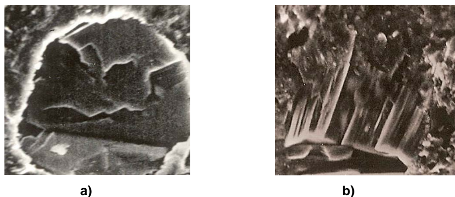
Figure 4. Microstructure of a modified low clinker binder, x2500 a – micropores of cement stone are compacted with thin sheets with CSH foil (1) (at 180 days of hardening age); b – Intergrowth of portlandite blocks with gel-like CSH.
