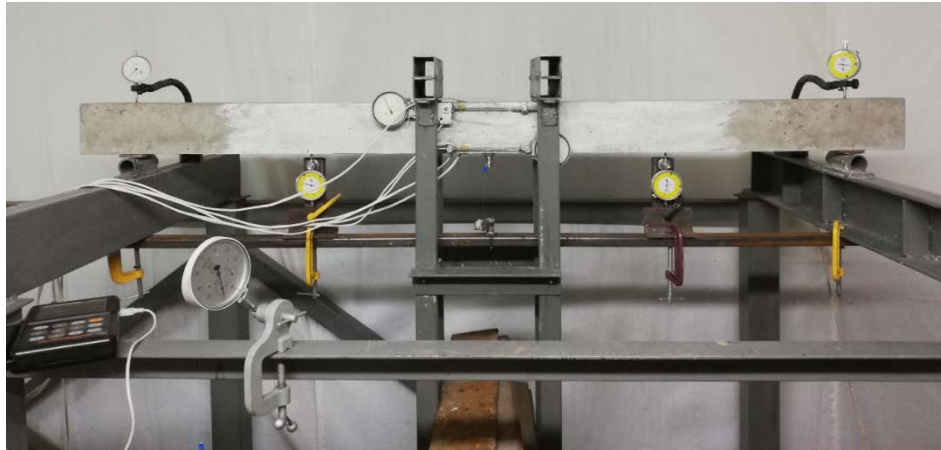
Figure 7. General view of reinforced concrete beams test before failure.
