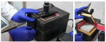
c - determination of the thermal conductivity of reference specimens
