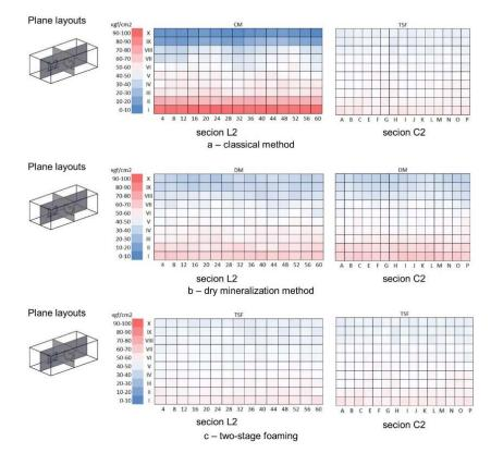
Figure 7. Color diagram of strength distribution in the cross-sections of C2 and L2 unit.
