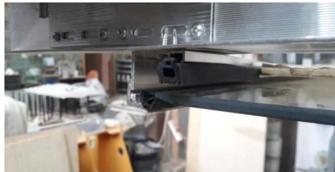
Figure 30. Residual deformation of profile after unloading (test setup 1).
