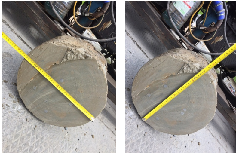
Figure 10. Diameter of drill-injection pile “N-1” after extraction.
