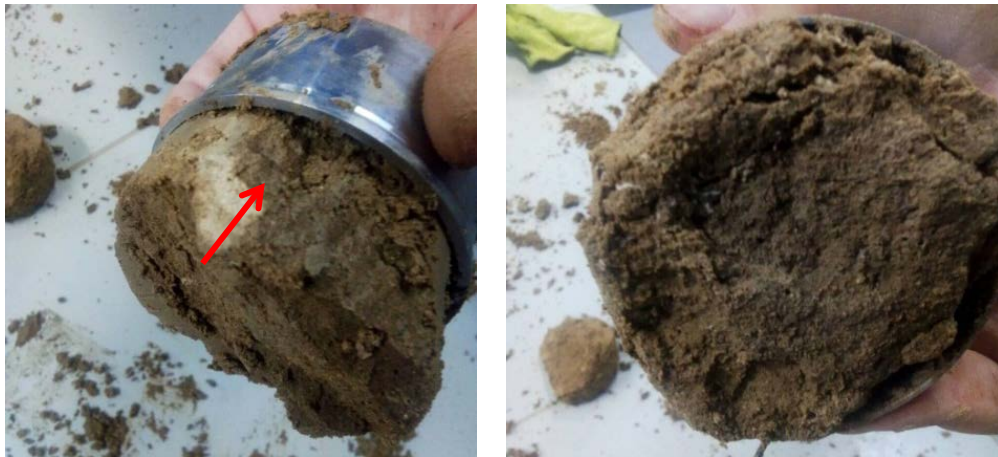
Figure 6. Cement particles incorporation into the range of the cutting ring No. 1.
