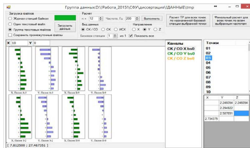
Figure 10. Interface of the “Standing Wave Method” program. Construction of phase diagrams of natural vibrations. Forms of natural vibrations.
