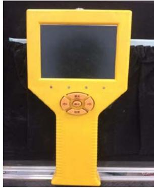
Figure 1. PTS-C10 intelligent crack width observer.
