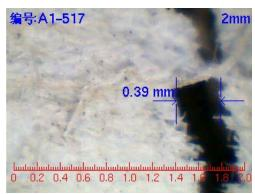
Figure 2. Crack width observation reading viewport.
