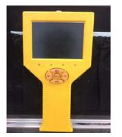
Figure 1. PTS-C10 intelligent crack width observer.
