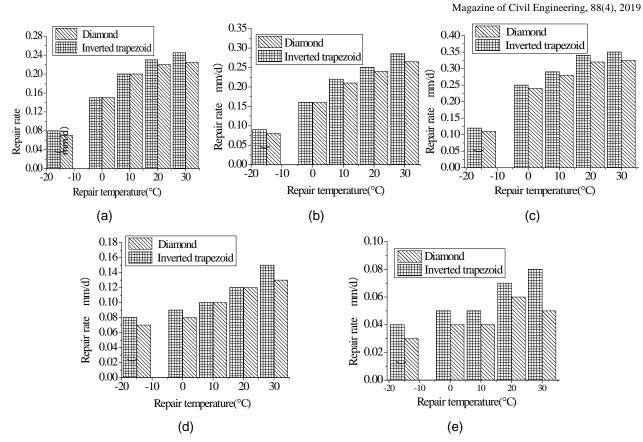
Figure 12. Change in repair rate as the fiberglass tube is placed:a) Initial crack width is 0.4mm; b) Initial crack width is 0.6mm; c) Initial crack width is 1.0 mm; d) Initial crack width is 1.5 mm; e) Initial crack width is 2.0mm.
