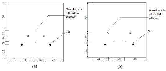
Figure 3. How to place the glass fiber tube in the test piece:(a) the glass tube is placed in a diamond shape (b) the glass tube is placed in an invertedtrapezoid.
