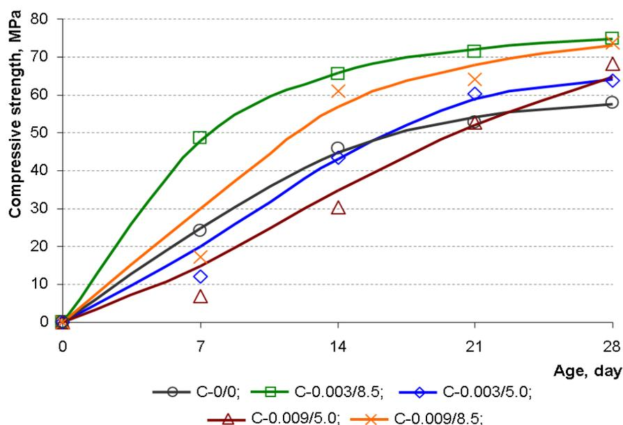
**Figure 2. Kinetics of hardening cement stone with SAP.**
