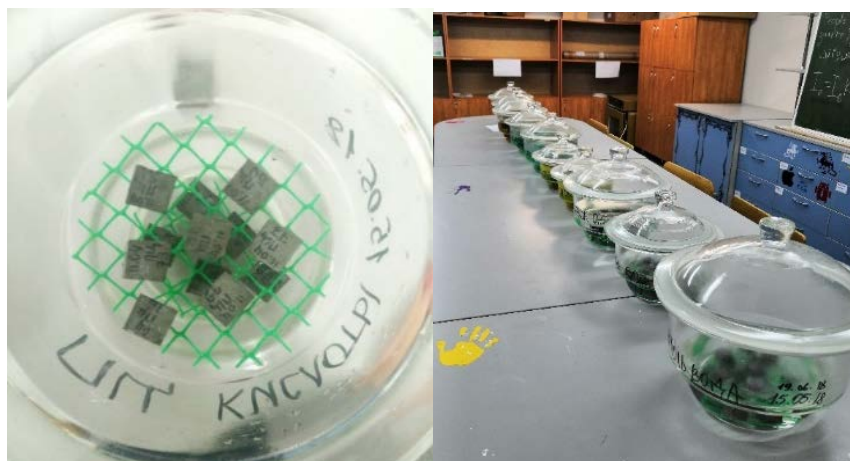
Figure 1. System for laboratory exposure of samples in model environments.
