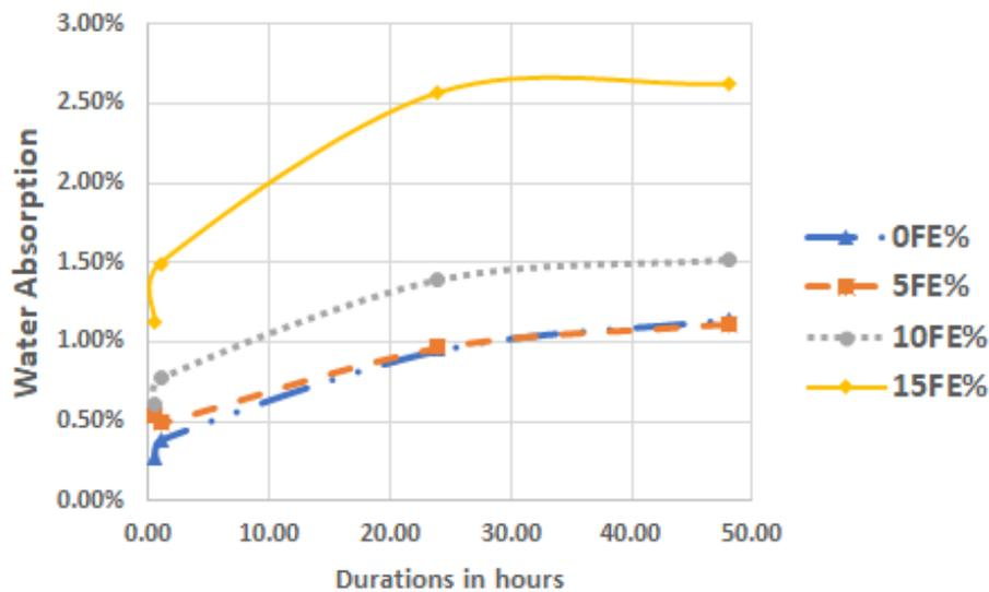
Figure 5. Water absorption based on the composition of iron-filing in paste.
