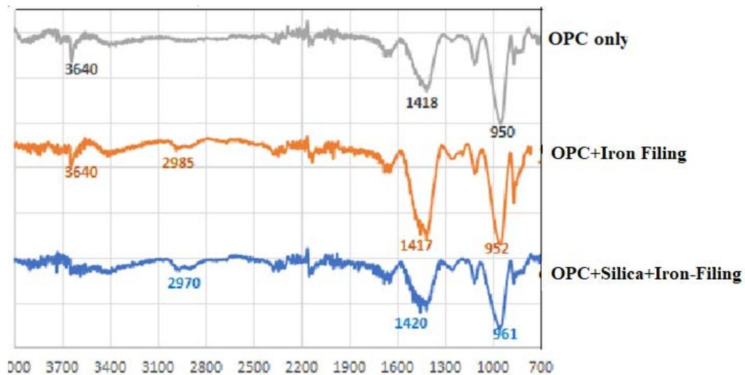
Figure 10. FTIR spectra (a) OPC only (b) OPC+10 %Fe (c) OPC+15 %Fe+10 %Si.
