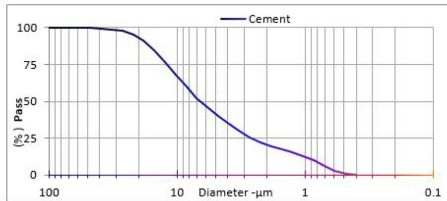
**Figure 1. Particle size distribution of the ordinary Portland cement.**
