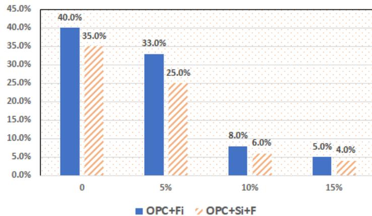
Figure 3. Workability of the paste with the presence of silica fume and iron-filing.
