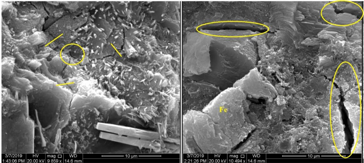
Figure 9. Micrographs of OPC paste (left) and OPC-Iron filing paste (right).
