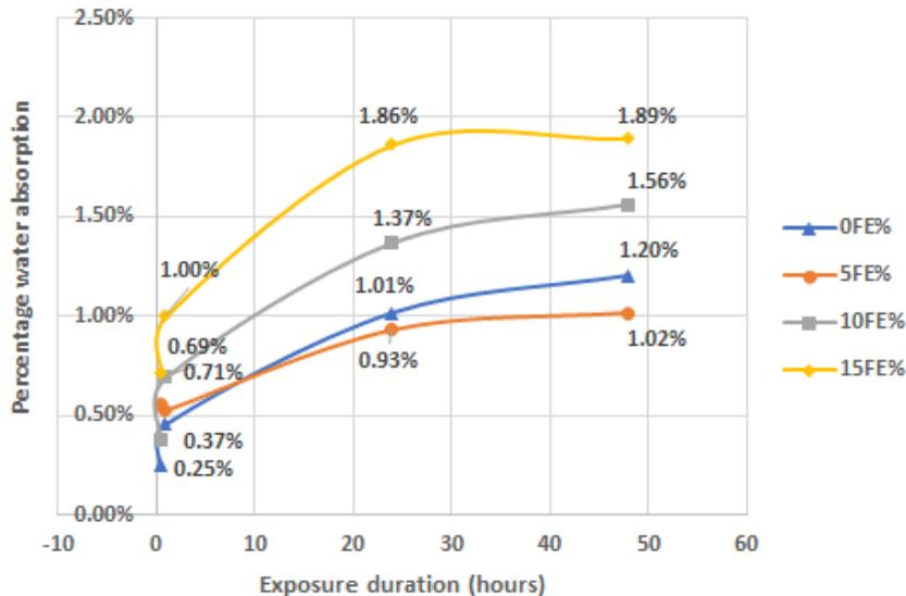
Figure 6. Effect of varied composition of iron-filing and silica fume (10 %) on the paste water absorption.
