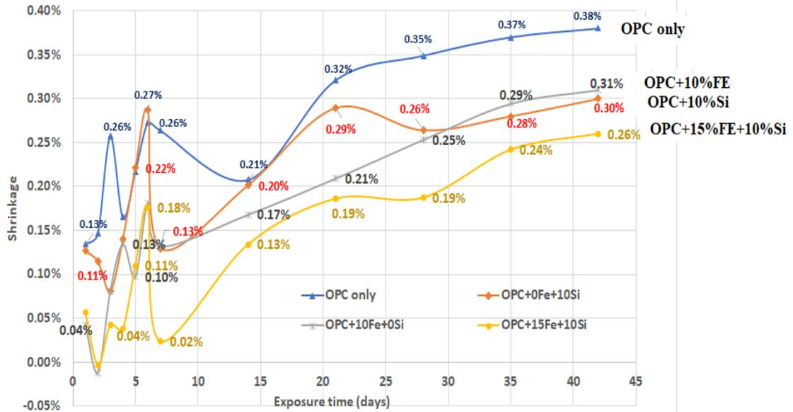
**Figure 11. Impact of silica and iron-filing on the shrinkage of OPC paste.**
