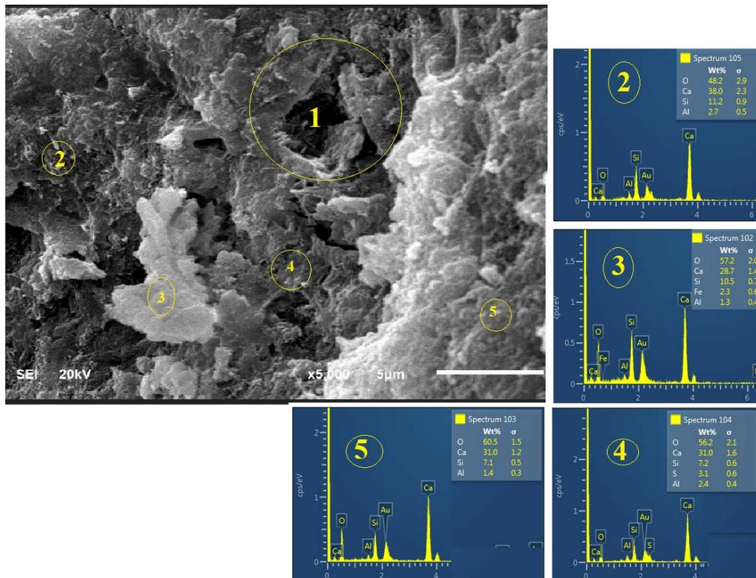
Figure 12. The micrograph of 10 %Si+OPC+15 %Fe.
