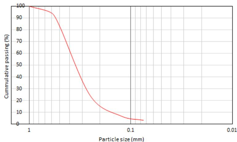
**Figure 2. Particle size distribution curve of iron-filing powder.**
