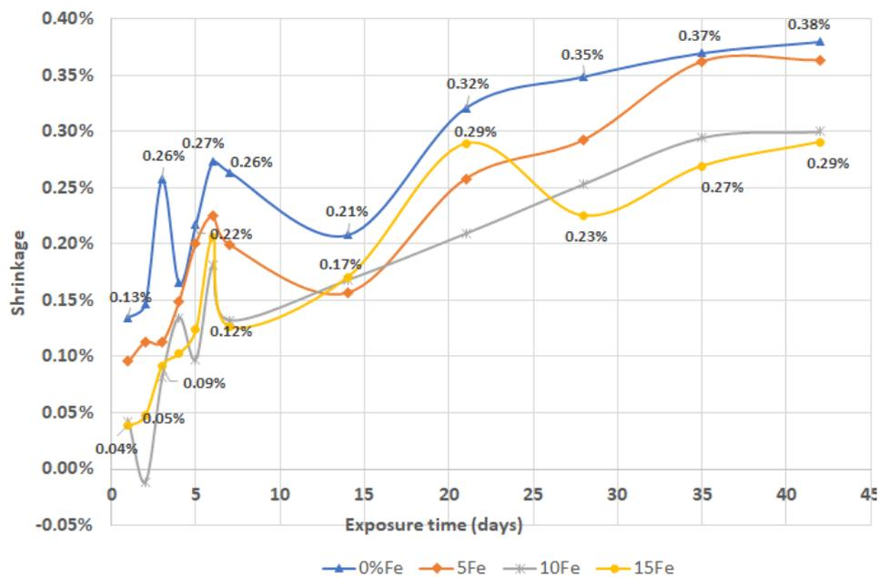
Figure 8. Shrinkage performance of iron-filing infused paste.
