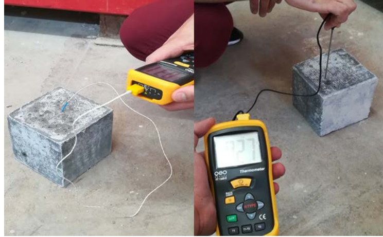
Figure 3. Photograph of a typical cube specimen with thermocouple used at the surface and centroid of the cubes.
