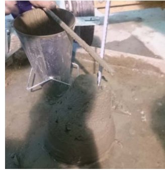
Figure 5. Control mix slump.
