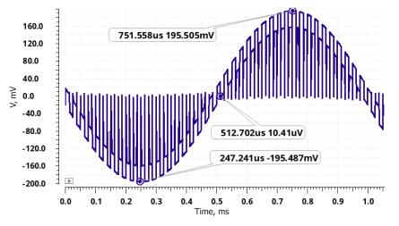
Fig. 6. Chopper amplifier's output signal
