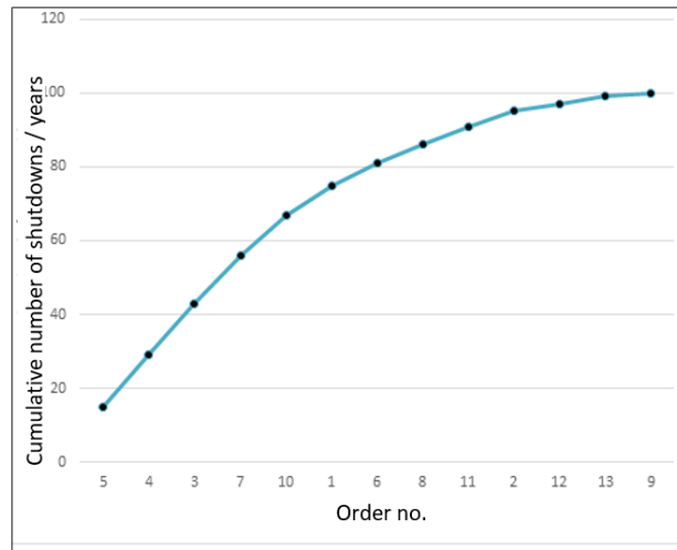
Fig. 3. The interventions on the drills of the machining workshop by the ABC method
