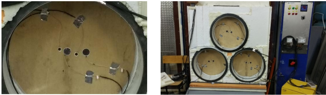
Figure 4. Experimental determination of thermal conductivity of foam glass gravel in a dry state at various degrees of compaction.
