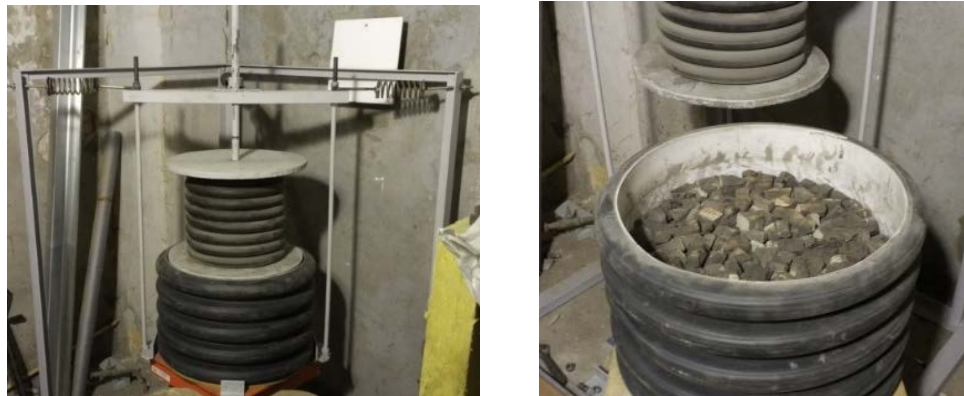
Figure 2. Carrying out experimental determinations of the maximum degree of compaction of foam glass gravel.
