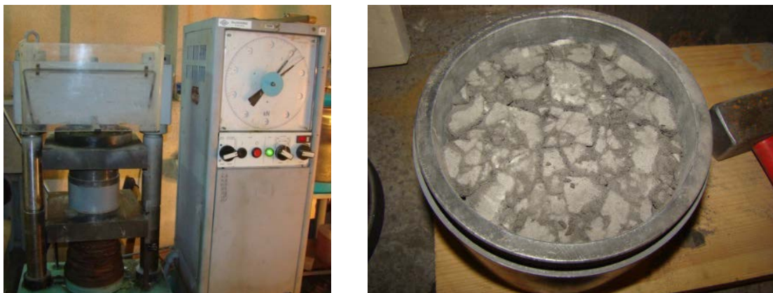
Figure 3. Experimental determination of the compressive strength of foam glass gravel at different degrees of compaction.
