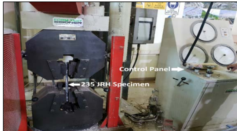
Figure 3. Experimental setup for coupon tensile strength testing.
