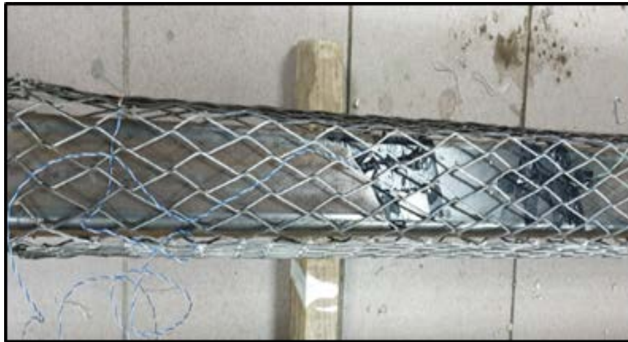
Figure 5. Steel mesh wrapping around the steel tube.
