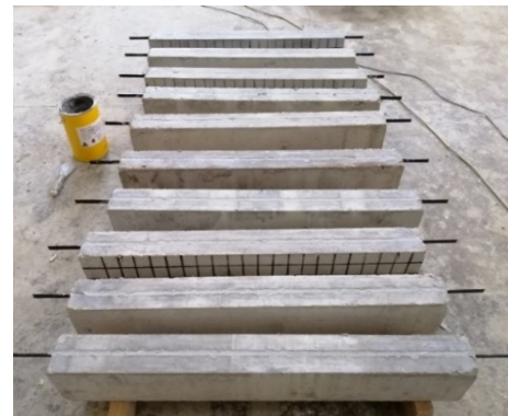
(f) Strengthened/Repaired beams
