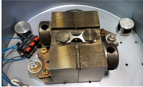
**Fig. 1.** Testing setup for thermal fatigue experiments
