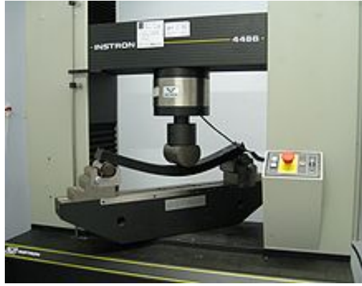
Fig. 6. Bending fatigue machine: INSTRON 4400
