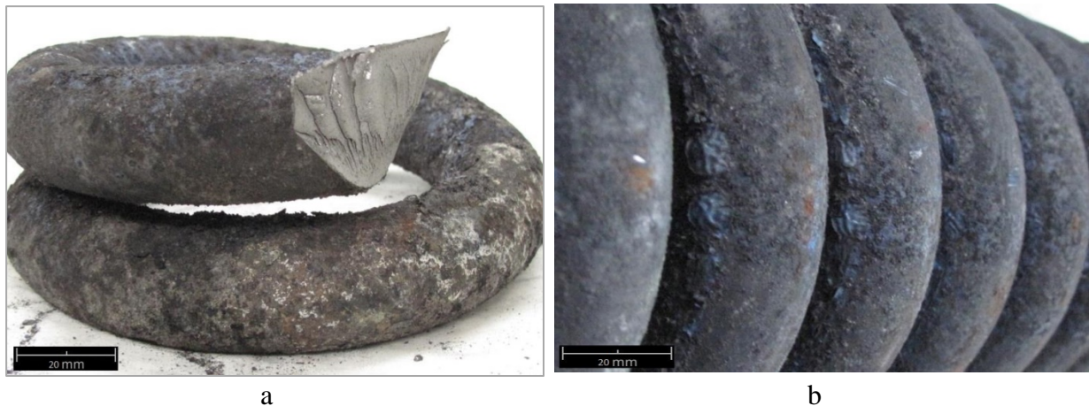
Fig. 1. Fragment of spring after failure: a – fracture surface; b – defects in the protective coating
