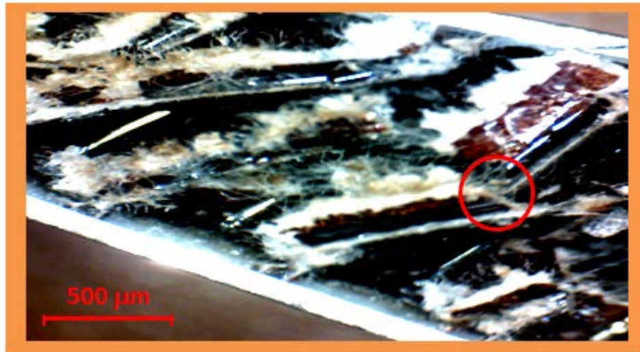
Fig. 10. Shearing of the core walls
