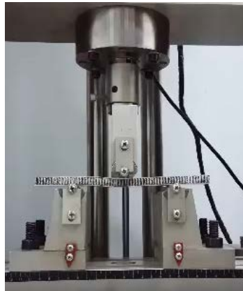
Fig. 4. Static bending test machine: Universal Machine WDW-5
