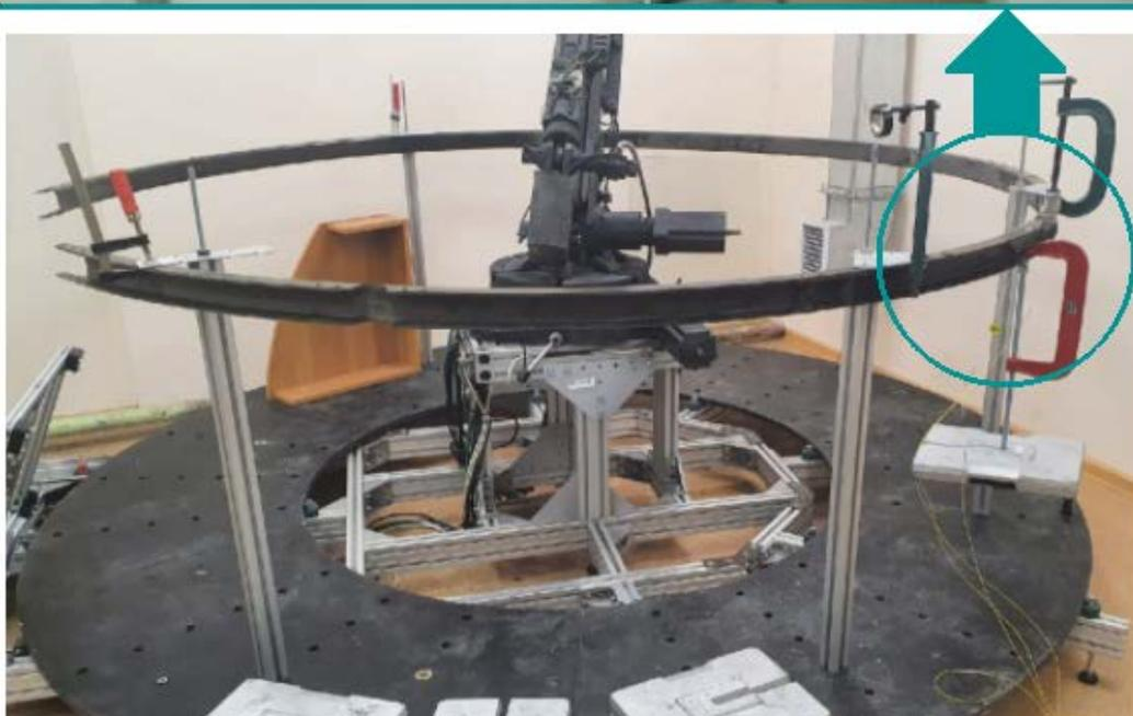
**Fig.6.** Mechanical test of the bulkhead. FOS placement scheme and application of load to the bulkhead segment center
