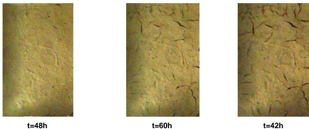
Figure 10.c cracks pattern evolution by drying (reinforced specimen \eta_f = 0.5 \% )
