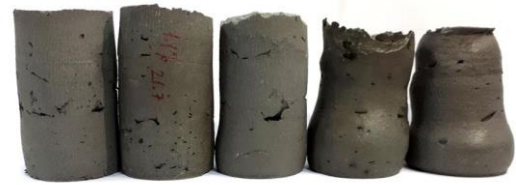
Figure 4. The nature of the slump of the concrete mixture after extrusion from the cylinder.
