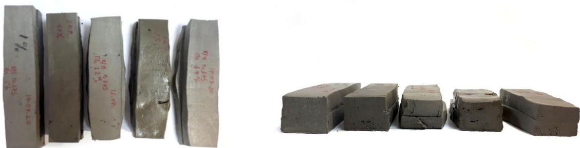
Figure 5. An example of deformations of extruded lightweight concrete layers in the horizontal (left) and vertical (right) planes.
