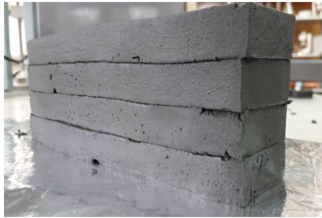
Figure 6. Example of extruded lightweight concrete layers with SAP.
