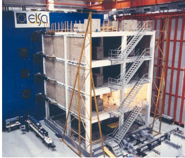
Figure 8. Four-storey 3D infilled frame tested by Negro et al. (1996) [29].
