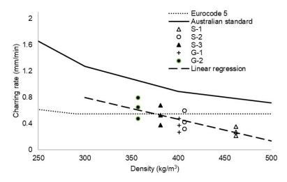
Figure 8. Comparison charring rate with other standard.
