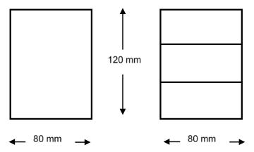
Figure 1. Solid and glulam cross section.
