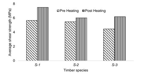
Figure 9. Shear strength comparison.
