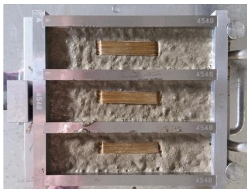
Figure 1. Preparation of the samples with steel wires for the controlled crack creation.
