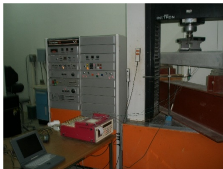
Figure 4. Measurements of the strains in reinforcing bars and the deflection at mid span using data logger.
