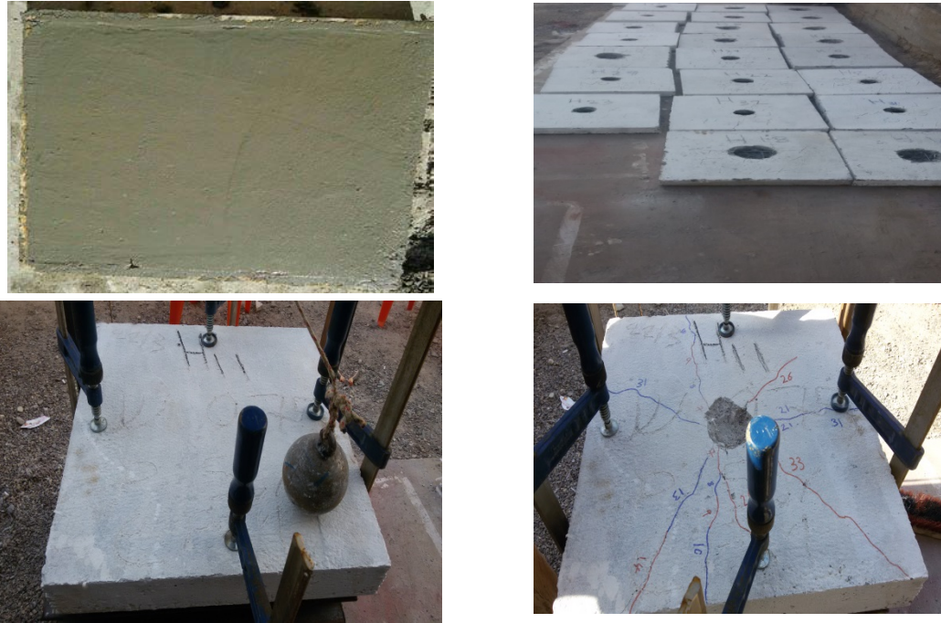
Figure 5. Failure of composite slabs under Impact force.
