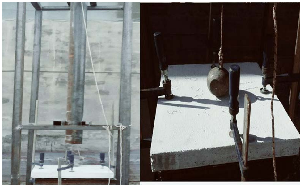
Figure 2. Frame test for impact loading.
