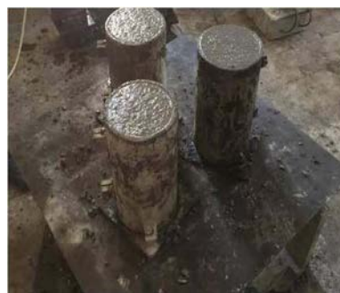
Casting concrete into cylinders
