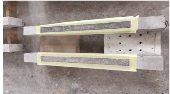
Concrete bonded area were roughened and brushed with steel wire cup brush
