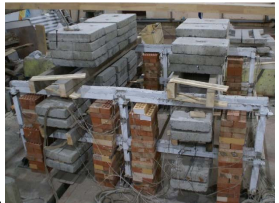
Figure 1. Experimental frame: a – the scheme of reinforcement of the combined part of the beams; b – the junction of the crossbar with the column at the 1 st stage; c – the junction of the crossbar with the column at the 2 nd stage; d – design diagram at the 1 st stage; e – design diagram at the 2 nd stage; f – frames photo at the 1 st stage; g – frames photo at the 2 nd stage.
