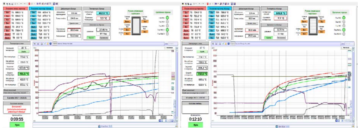
Figure 4: Graphic of temperature changes at thermocouples (monitor of test equipment TIZOL JSC): Red – upper limit of temperature deviation tolerance from ISO curve; Blue (dark) – lower limit of temperature deviation tolerance from ISO curve; Green – set temperature in the furnace; Black – actual average temperature in the furnace; Blue – average sample heating temperature.
