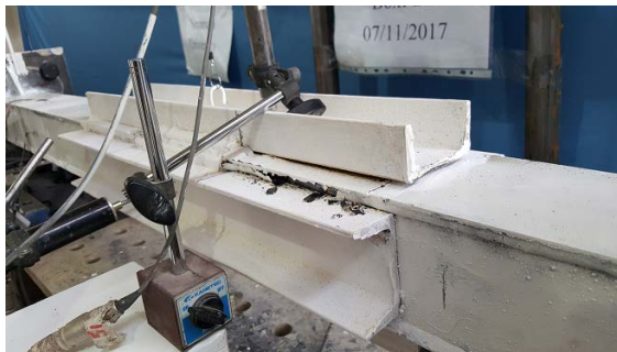
(a) prevention of fuse local buckling by auxiliary elements
