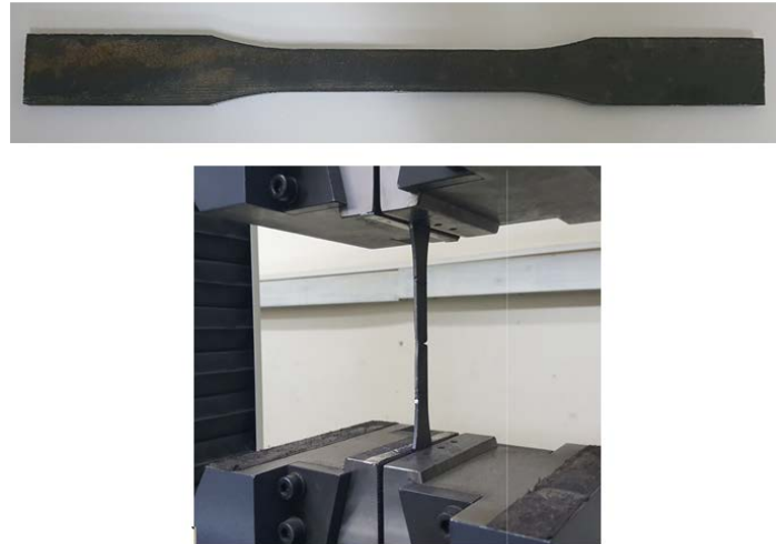
Figure 17. Standard tension test of steel material (based on the ASTM E8 standard).
