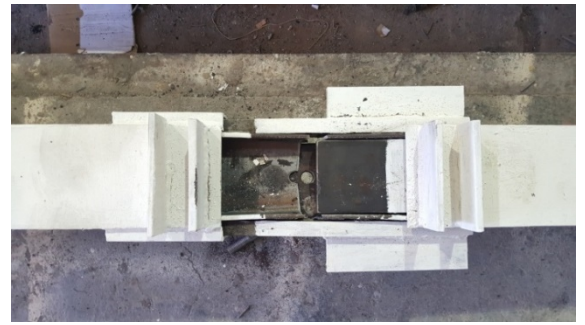
(b) tearing of the brace in the middle of the fuse
