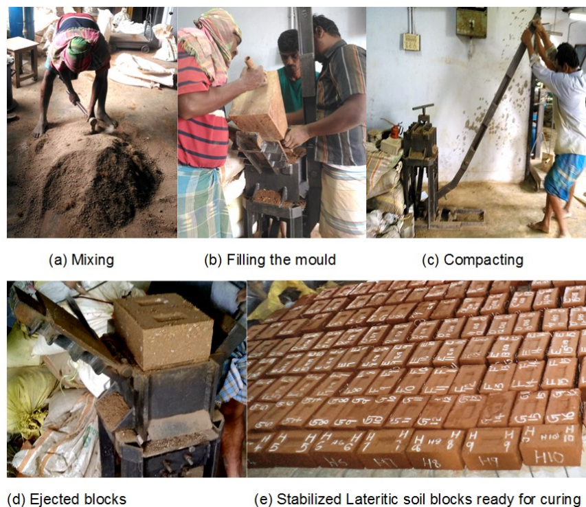
Figure 2. Manufacturing process of Stabilized Lateritic soil block specimens.
