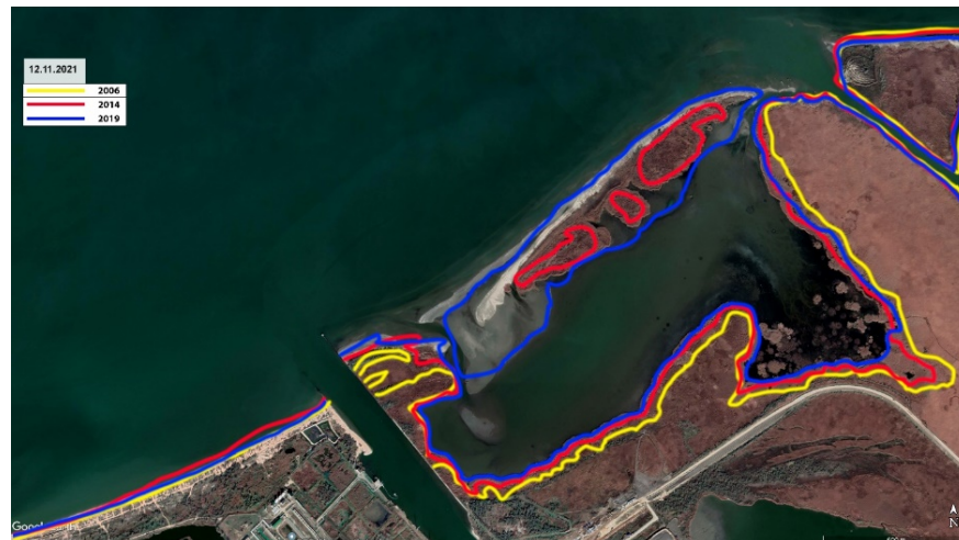
Figure 12. Shoreline changes in the area of the channel mouth from 2006 to 2019 based on the analysis of satellite images.
