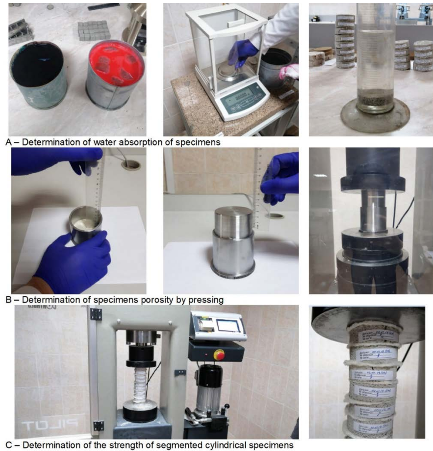
Figure 3. Laboratory testing of foam concrete specimens.
