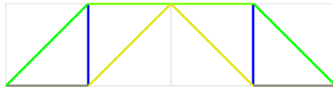
Figure 9. Resulting truss topology.
