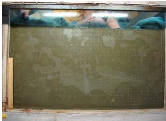
Figure 3. General view of the laboratory setup window with deformation benchmarks placed in the initial position.
