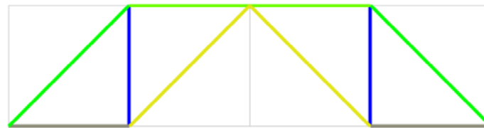
Figure 9. Resulting truss topology.
