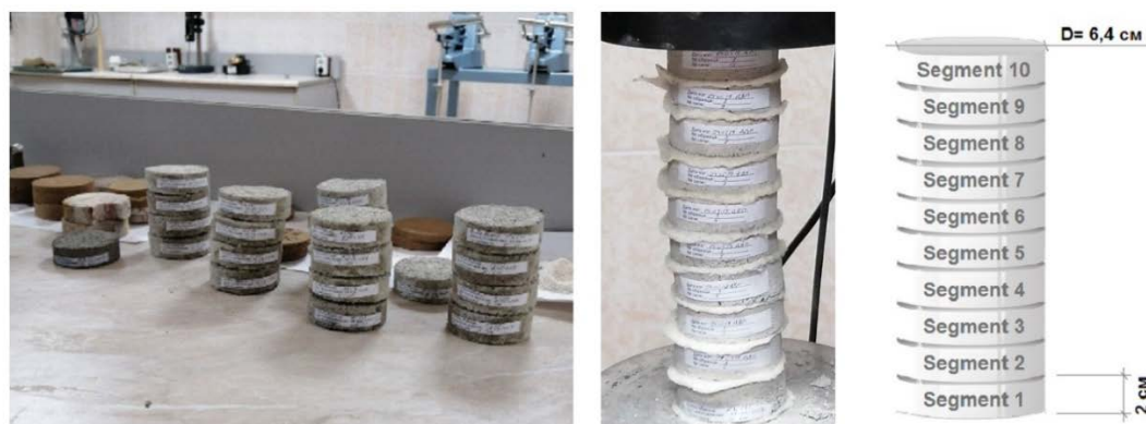
Figure 2. Specimens for determining the construction properties of foam concrete.
