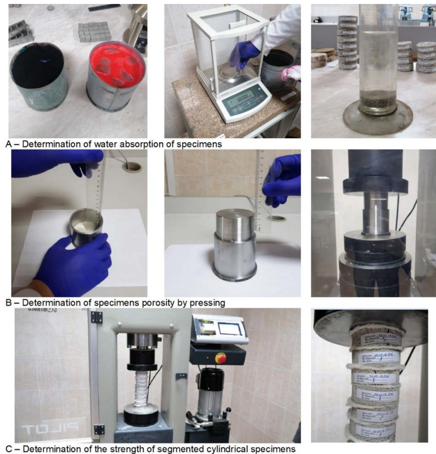
Figure 3. Laboratory testing of foam concrete specimens.
