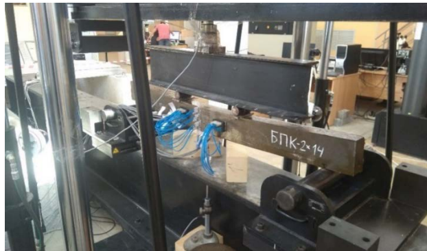
Figure 5. General view of the beam BRR-2x14 prepared for testing.
