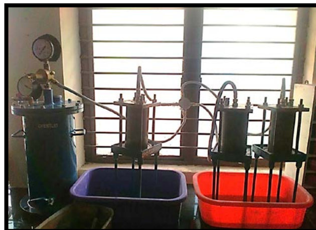
Figure 6. Test setup for Water permeability.
