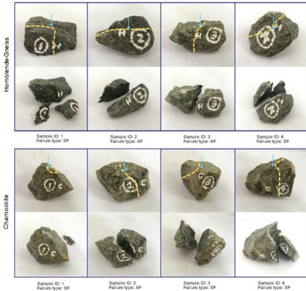
Figure 9. Failure planes of typical rock specimens with respect to load applied (SF: Shear failure; AF: Axial failure).
