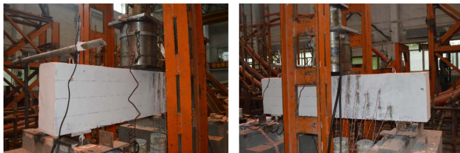
Figure 3. Mesh and strain gauges on the surface of the RC-control beam.
