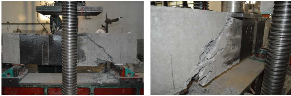
Figure 6. Failure mode of the RC beam strengthened with basalt fiber sheets.
